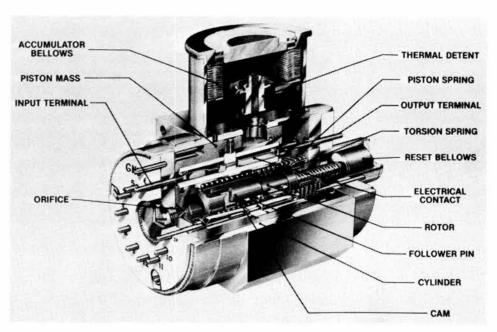
ENVIRONMENTAL SENSING DEVICE is the first to be actuated by two acceleration-time pulses. It provides abnormal-environment safety for the W87/MX.
